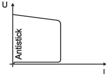
**The Antistick feature prevents the electrode from annealing.** Should the electrode stick, the machine automatically switches to the minimum current within approx. one second. This prevents the electrode from annealing. Check the welding current setting and correct for the welding task in hand.
